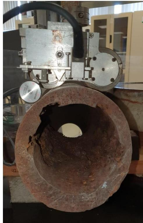
**The orientation and position of the transducer is necessary to properly shot the transducer and reconstruct a 3-D model of the specimen**
