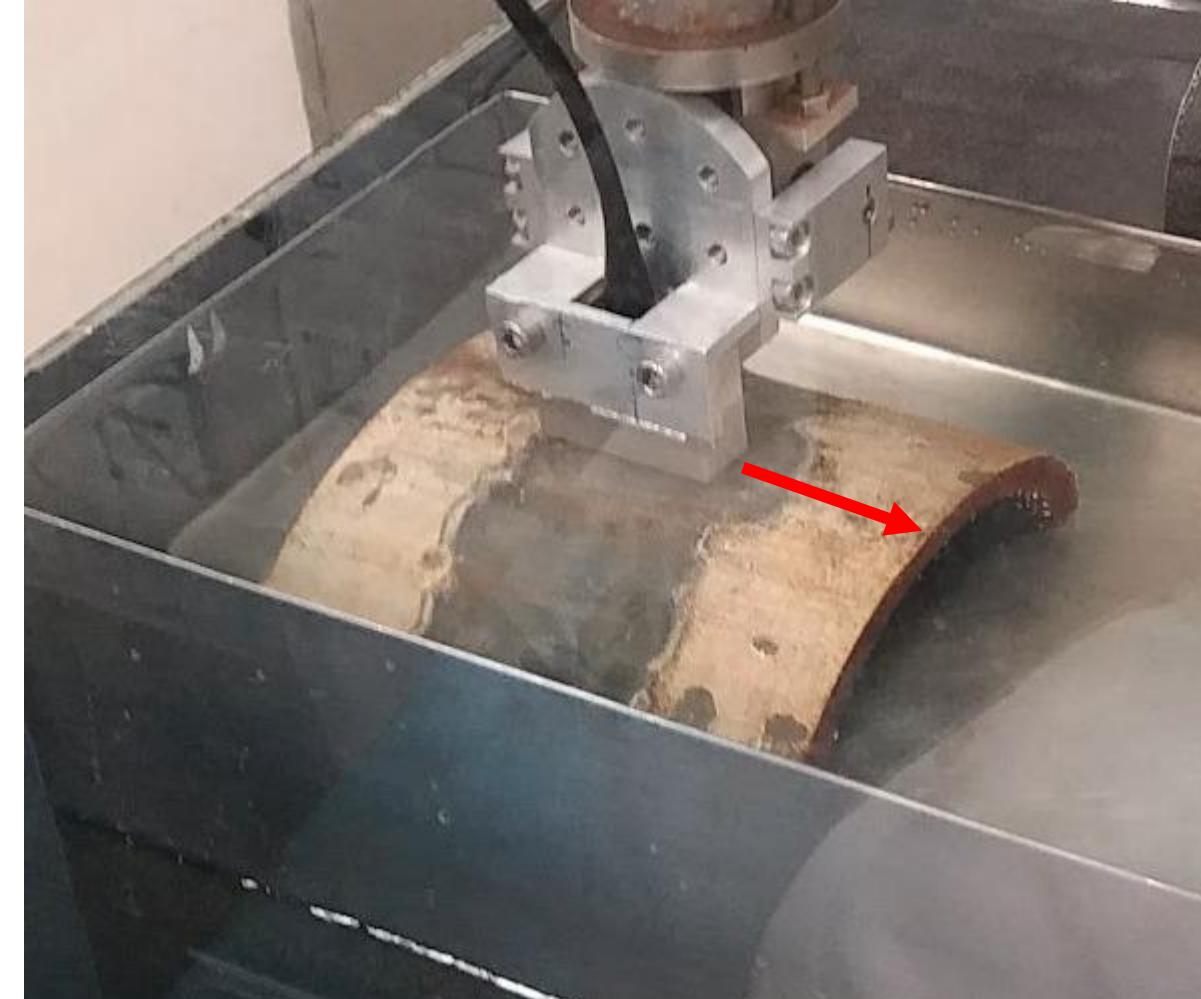
**The orientation and position of the transducer is necessary to properly shot the transducer and reconstruct a 3-D model of the specimen**
